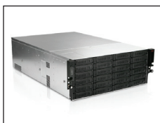
EX4M36-EXP 4U 36-Bay Storage Server Rackmount Chassis with SAS Expander
